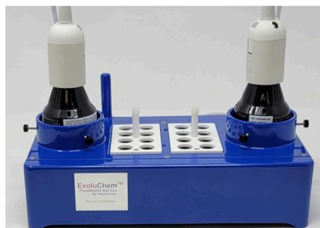
This photoreactor with double-capacity leverages the same patented concept (US Patent #10,906,022) as the original PhotoRedOx Box™. PhotoRedOx Duo™ increases the reaction vials capacity to 16 vials (2, 4 or 8 ml) using 2 of the same vial holders as the PhotoRedOx Box™. Using the 2 LED setup allows to increase reaction rate of difficult reaction conditions.
