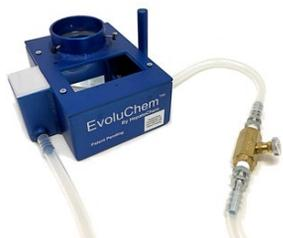
All the benefits of the PhotoRedOx Box™ with temperature control from 0°C to 80°C. The unique reaction chamber geometry directs light throughout, allowing the performance of multiple reaction conditions simultaneously. However, with the aluminum-based, waterproof PhotoRedOx TC™, it is possible to heat and cool the reaction medium using a thermostatic fluid (such as water or ethylene glycol) that recirculates through a standard chiller/heater unit.
