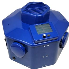
This photoreactor is designed to perform photochemical reactions using UV and Visible light from 254 nm to 808 nm. It is compatible with holders for 8X 4 ml vials, 8X 8ml vials and 4X 20 ml vials. The reaction temperature is monitored using an IR probe and regulated with internal fans. This photoreactor comprises a stirring module and user interface to setup the experiments.
